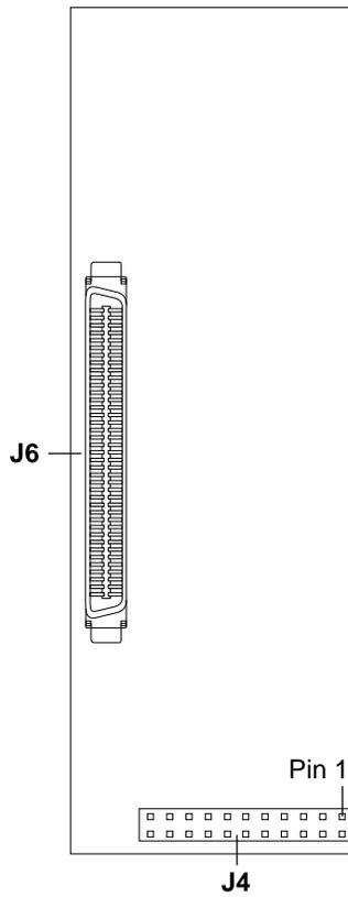
Figure 24. ST15150WC/DC drives option select connectors
