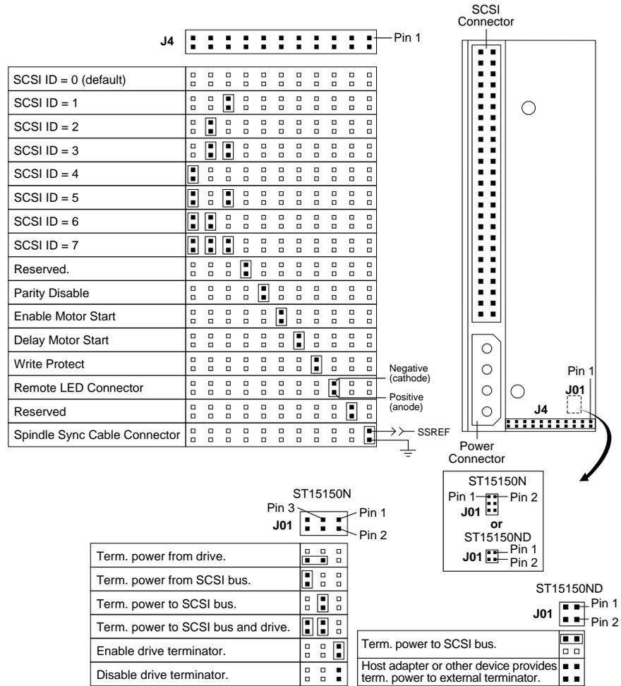
Figure 20. ST15150N/ND drives option select jumper connectors
