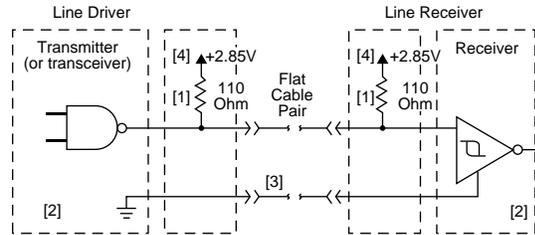
**Figure 31. Single-ended transmitters and receivers**
