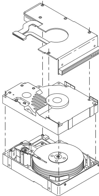
Figure 2. Barracuda 4 disc drive (exploded view)
