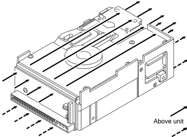
**Note.** Air flows in the direction shown (back to front) or in reverse direction (front to back)
