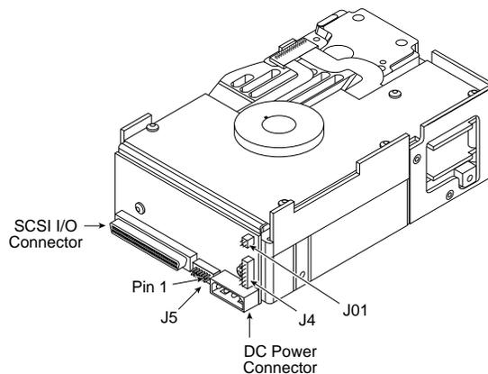
**Figure 29. ST15150W/WD drives physical interface**
