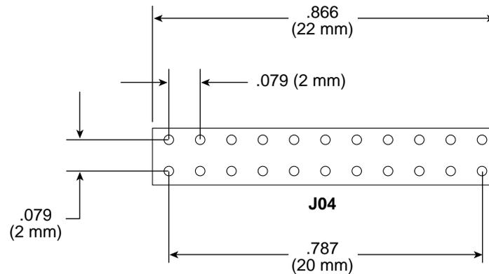
**Figure 26. ST15150N/ND drives configuration select header specification**
