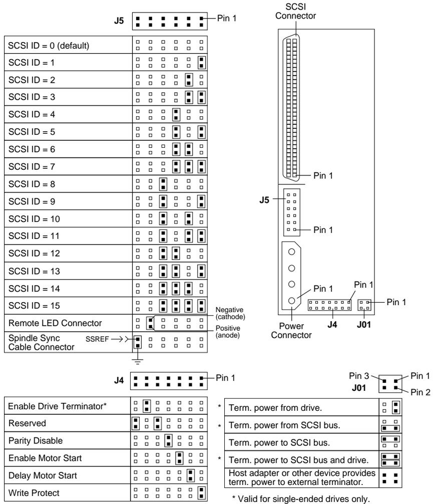
Figure 22. ST15150W/WD drives option select jumper connectors
