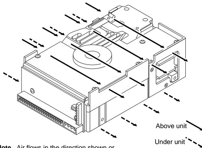
**Note.** Air flows in the direction shown or in reverse direction (side to side)
